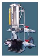
This swimming pool portable vacuum filter uses a 1HP, 110 VAC, Sta-Rite Dyna-Max pump to move approximately 5400 gallons of water per hour through a 155 square foot Harmsco stainless steel cartridge filter. Also available as gas powered if an outlet is not available. your pool floor.
